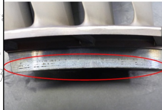
GEnx-1B/2B LPT Stage 1 Nozzle - Update of Serviceable & Repairable Limits
